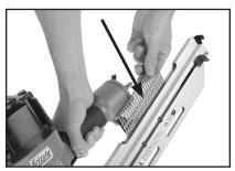
Figure 4. Loading nails into magazine.
